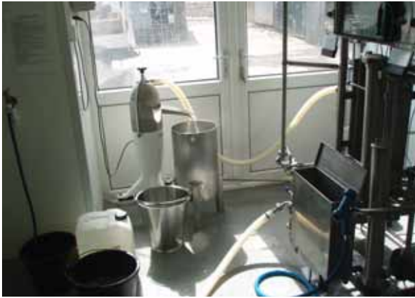
Unit separating the cream from the milk. Source: C.E. Lloyd Swansea University
